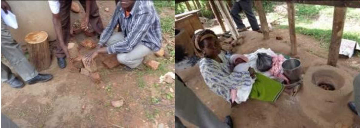
Left: Jasper and Isaac showing the curved bricks they use for making jikos
