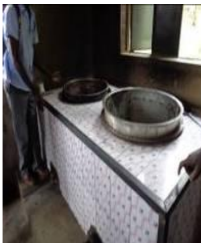
Extreme left: a smoky cooking pan loaded on an energy saving jiko; Middle and extreme Right: Improved smoke free energy saving jikos used by the school, using smoke preventing pan
